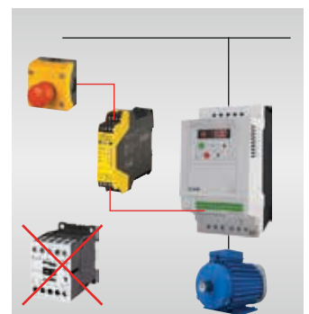
The built-in STO (Safe Torque Off) safety function makes a mains contactor unnecessary.
